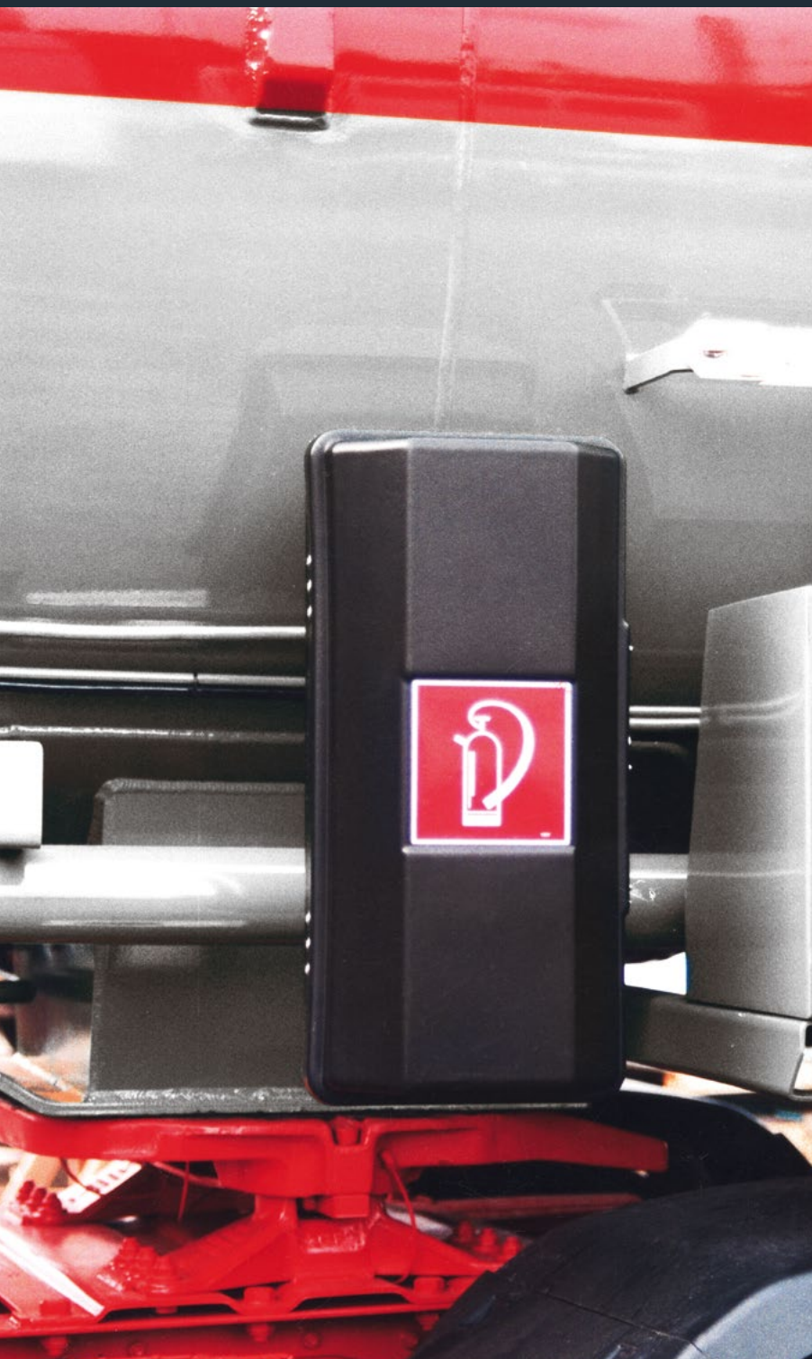
Fixture for vehicle mounting made from red painted steel
